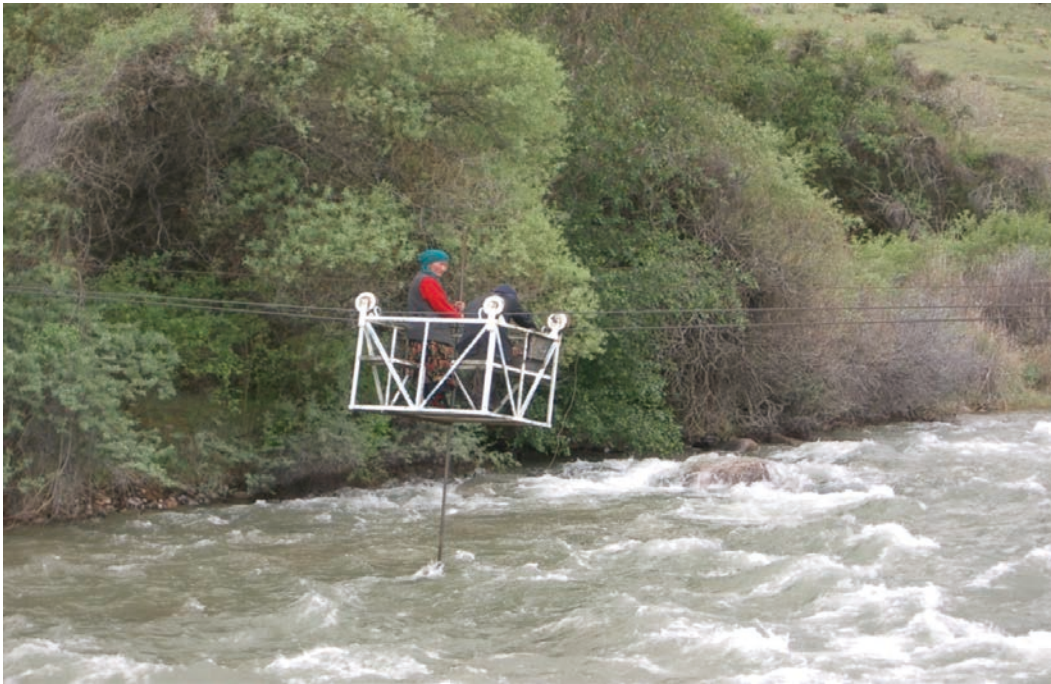
Figure 26. In-stream flow measurements can be a hazardous occupation under flood conditions. Each year accidents associated with this type of flow-velocity sampling occur. (Courtesy: USGS.)
