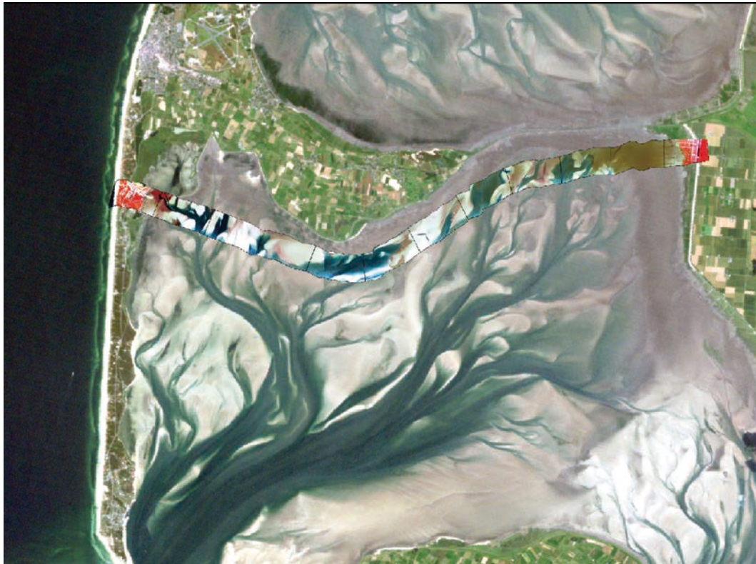
Figure 38. Satellite scene (Landsat TM) with low spectral resolution from the northern German Wadden Sea with an hyperspectral overlay from an airborne instrument. Currently no data are available for such a highly structured region of water and intertidal areas with full spectral information on rapidly changing water contents and bottom coverage. This will be available with the German hyperspectral satellite Environmental Mapping and Analysis Program (EnMAP) as it delivers the spatial resolution of Landsat/TM or Sentinel-2 with the full spectral information from 420 nm to 2,450 nm like airborne systems. (© Copyright Helmholtz Zentrum Geesthacht 2013.)
